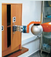
Velma robot opening the door
